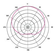
Directivity: Uni-directional Output connections: XLR (3-pin) Frequency Response: 50Hz - 14 KHz
